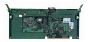
The XTS-IP In-Skin FLASH unit comes complete with 8 ports of voice mail and up to 64 mailboxes. The basic configuration comes standard with 3 hours of message storage, and can expand to 9 hours of storage with a memory expansion card.
