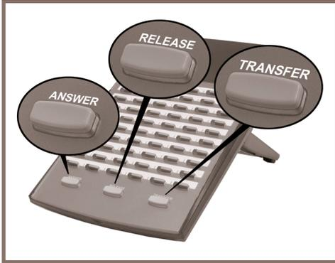
For more call handling power and flexibility, the DSS Console provides 60 additional Feature Keys as well as three Speed Processing Keys along the bottom. (For more on setting up Feature Keys, see the *Telephone Feature Handbook*.)
