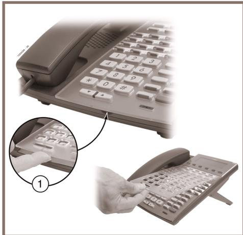
To remove the faceplate (if installing a custom DESI label):
