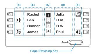
32 (8 keys x 4 pages) additional programmable keys are provided. They can be programmed as Flexible Line/Programmable feature key by Telephony Server Administrator. For the SV9100, the programmable keys can be set by WebPro/PCPro/Handset Pro and the user can also set them.
