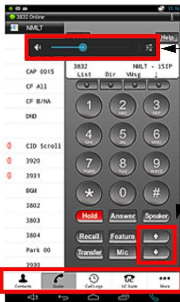
← The volume of the device is controlled by the PBX and the user can set the volume level with the up and down keys after selecting the voice key when the App is running. The change in volume will be set in the PBX as well as on the device. The device volume display reflects the current value set from the App.
