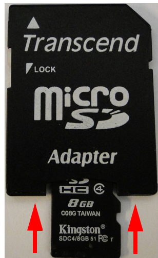
Figure 1-4 Inserting the “Micro SD” Memory Card into the Adapter
