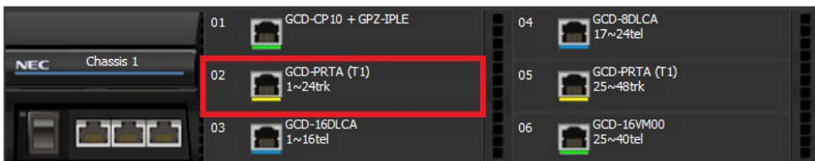
Figure 2-33 Digital Trunk Clocking Example 4
